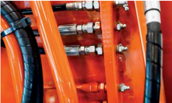
The centralised greasing point combines all five points in one for easy maintenance.
